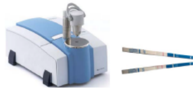
Fourier-transform infrared (FTIR) spectroscopy machine and immunoassay test strips.
